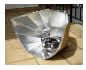
food is ready within 2-3 hours. The CooKit is made of cardboard, lined with aluminium foil. A lightweight 4-litre, flat black painted pan is placed in the CooKit, in a heat resistant plastic bag.
