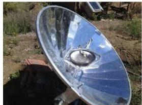
There are many designs for parabolic solar cooking appliances. Because of the parabolic shapes and with the aid of reflecting material quite a lot of solar energy is concentrated in the focal point. A very high temperature of between 200 and 300°C can be reached because of a combination of the circular design, the size and the polished aluminium. It is suitable for baking, roasting and grilling.
